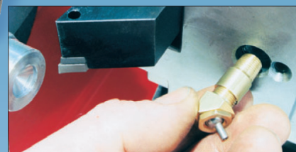
DualFit brass adaptor allows PressureMax nozzle to be used in screw-lock socket having BSPT port.
